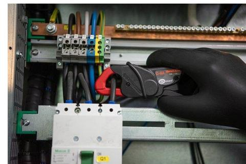
The gap (formed by the faces of the core) should be kept perfectly clean.
